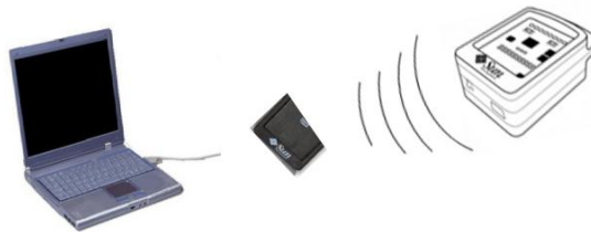
Figure 4. Elements of the accelerometer sensor network
